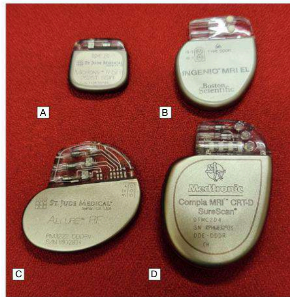
Fig. 16.51 Cardiac implantable electronic devices. A Single-chamber pacemaker. B Dual-chamber pacemaker. C Cardiac resynchronisation therapy pacemaker (CRT-P). D Cardiac resynchronisation therapy defibrillator (CRT-D).
